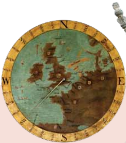
This beautifully intriguing object is positioned over the fireplace in the King's Gallery (pp20-21). Connected to a wind vane on the palace roof, the dial told King William III which way the wind was blowing and where his navies were likely to be.
